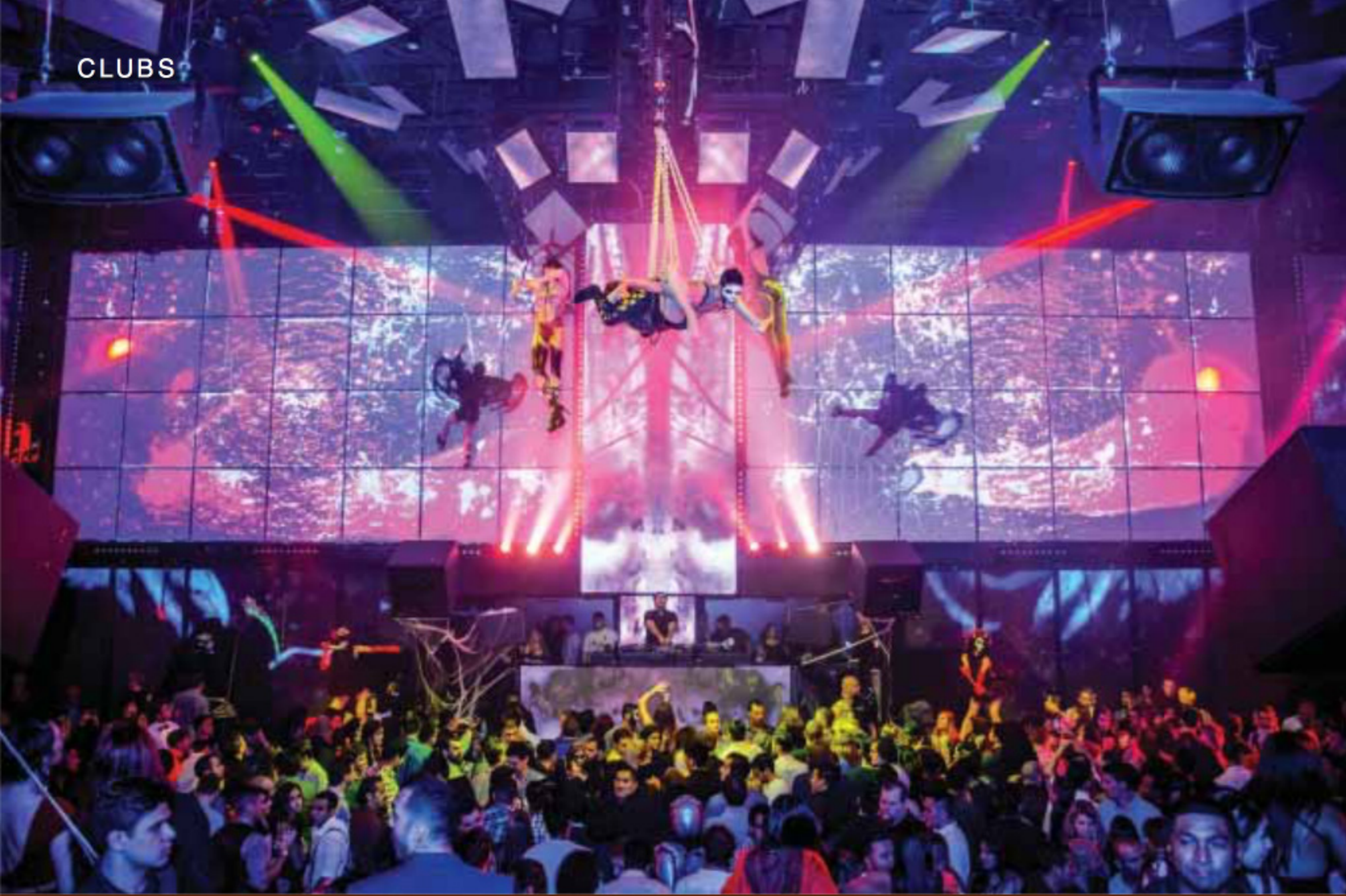
The acro walls on each side of the DJ booth are 20' tall by 30' wide and fitted with tiled Lexan polycarbonate panels covered with a white translucent 3M Scotchlcal perforated window graphic film.
